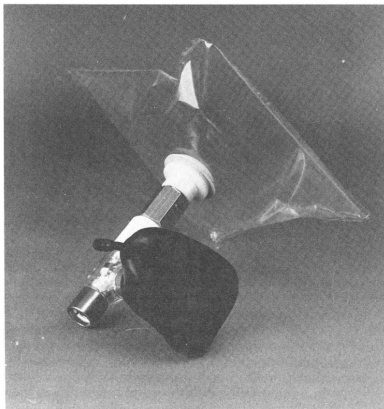
Fig. 1. The anesthetic mask equipped with a Ruben valve connected by means of a gas tight cock, to a polyvinylfluoride bag.
